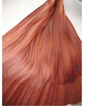
There are mastered production and sales of 12 standard grades of nylon cord fabrics that are of demand at tyre manufacturers as high quality goods. Among fabric grades being produced there is a special demand in fabric grades with lower surface density such as: 30 (302) KNTS-P from the yarn of structure tex 187x1x2 and 22 (222) KNTS-P from yarn of structure tex 144x1x2.
