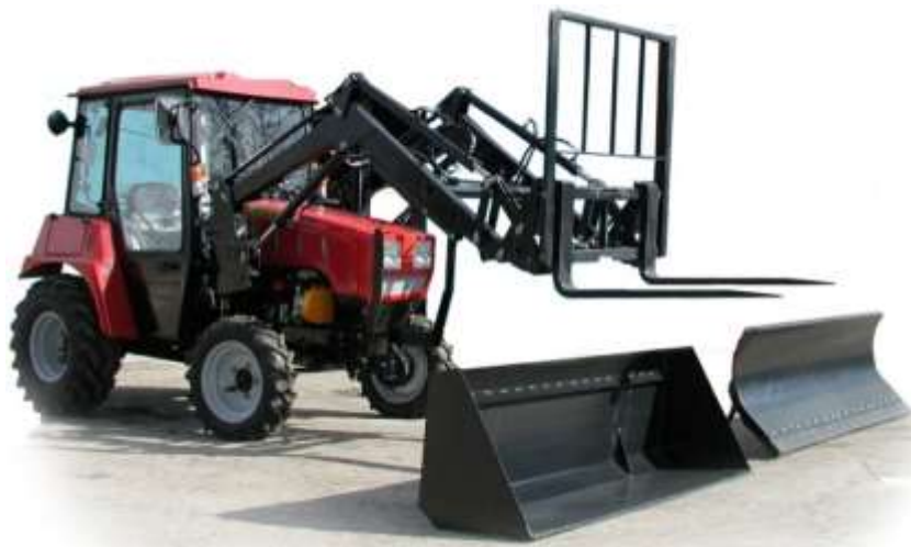
Loading equipment with replacement plants.
